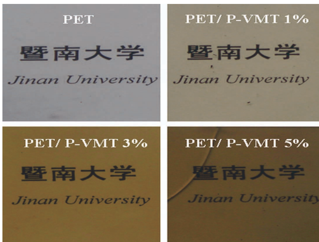
Figure 1 Visual appearance of the PET/P-VMT composites. [Color figure can be viewed in the online issue, which is available at wileyonlinelibrary.com .]
